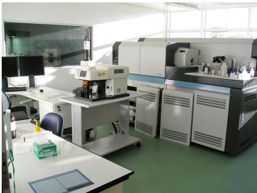
Figura 12 - LA-MC-ICP-MS (*Laser Ablation Multicollector Inductively Coupled Plasma Mass Spectrometer*) da marca Thermo Finnigan, modelo Neptune.
