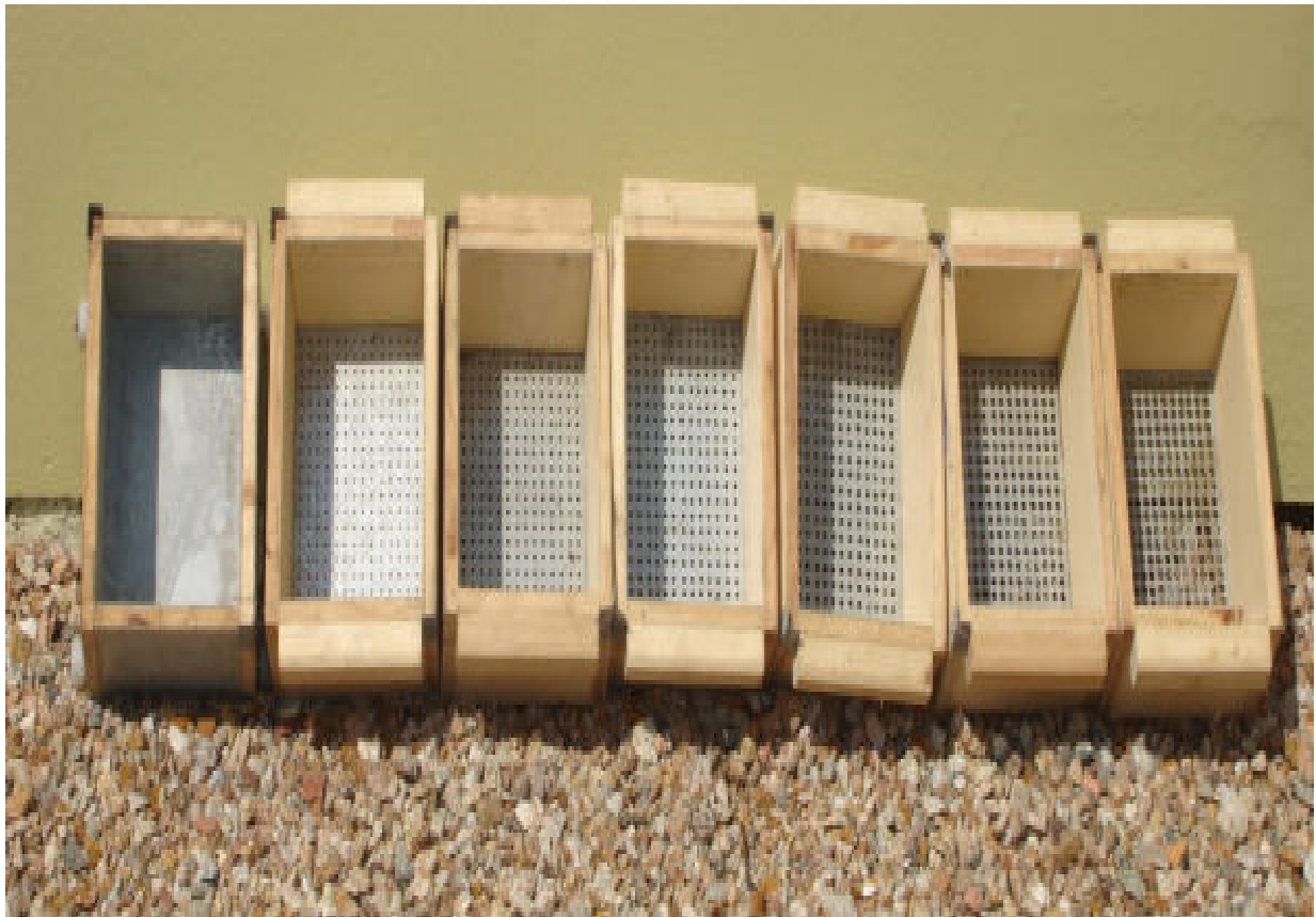
Figura 6.3: As peneiras de malha circular de < 2, 2, 3, 4, 5, 6 e 7 mm.
