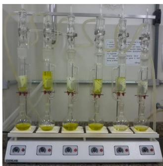
FIGURA 2: Extrator *Soxhlet*.
