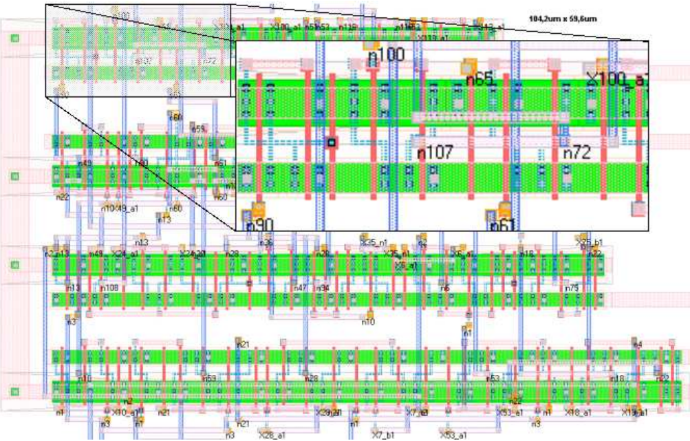
(b) Short polysilicon connections but big transistors drain/sources areas
