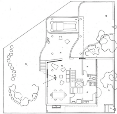
ground floor 1 garage, 2 living room, 3 veranda, 4 kitchen, 5 servant's room, 6 lavatory, 7 service court, 8 garden, 9 view
