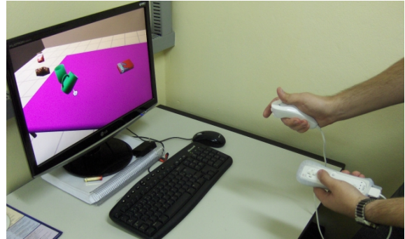
Figure 2. Using the Nintendo Wii Remote ® and Nunchuck ® to interact with the supermarket scenario. In this stage the Nunchuck ® is being used to rotate the selected object so its orientation can match the one of the fixed copy on the table.
