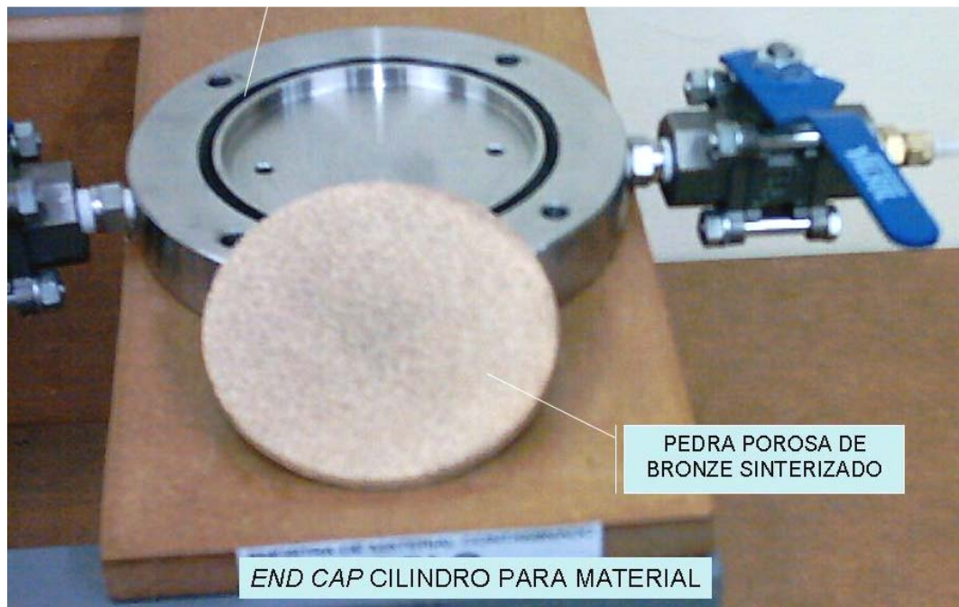
Figura 3.5 – End cap com pedra porosa e o-ring.
