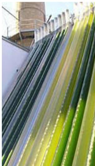
**Figura 6 - Fotobiorreator de coluna de bolhas no MIT (Massachusetts Institute of Technology)**
