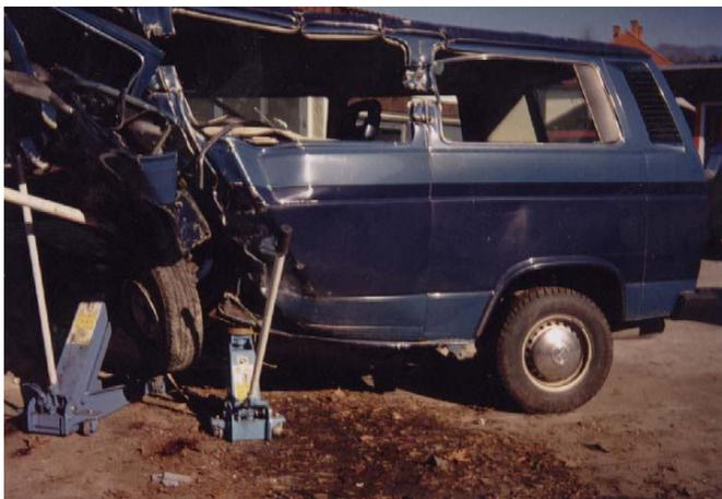
Figura 2.15 Danos causados na van VW Caravelle, Balazic et al., 2006
