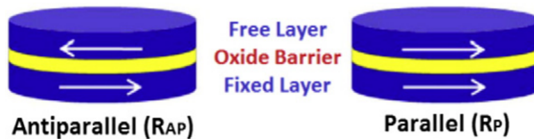
Figure 18: Magnetic tunnel junction (MTJ) structure and the two possible states of relative magnetization orientation.
