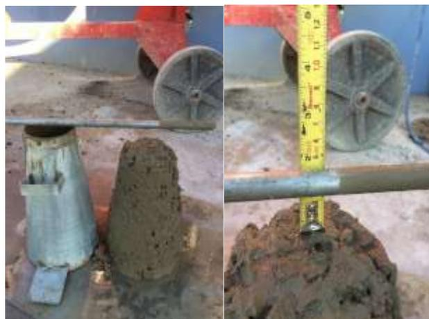
**Figura 6: Slump test.**
