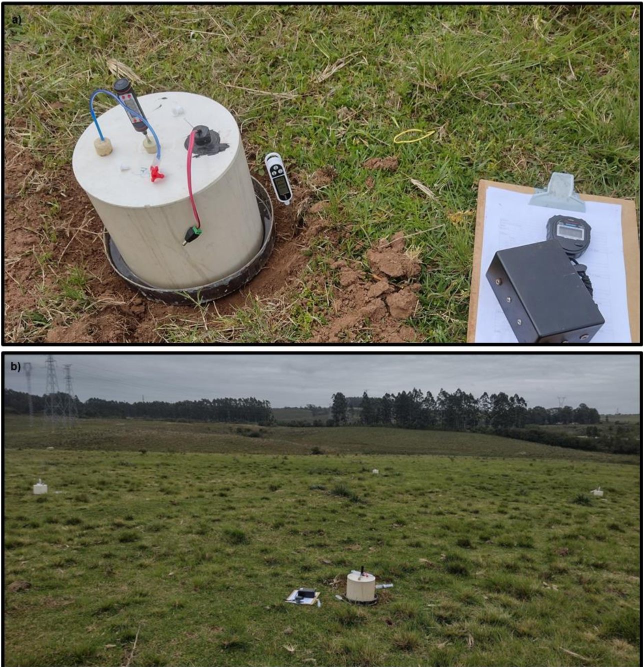
Fig. 3 Static chambers used in the soil gas sampling experiment. (a) Chamber installed with the metal base attached to the ground, with a digital thermometer to measure the internal temperature of the chamber, and a digital thermometer inserted into the ground to measure the soil temperature, a battery to power the internal fan and a three-way system to collect the gas using a syringe. (b) Four chambers installed at Point 3 - Ranch - UTE.
