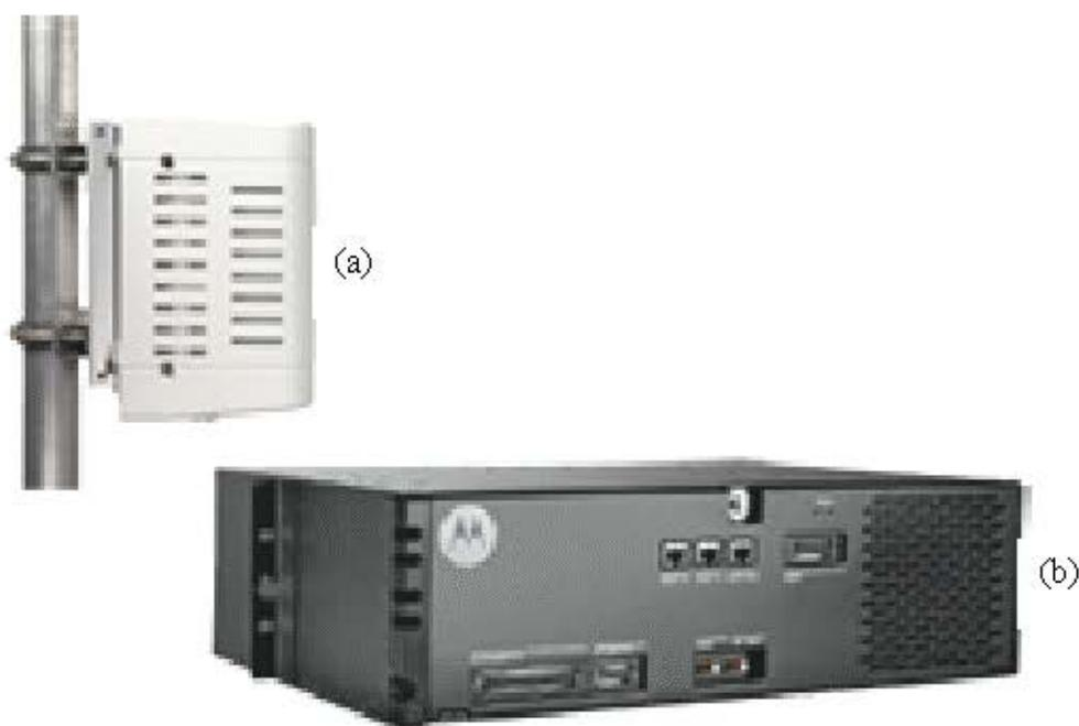
Figura 2.9: Equipamentos eNodeB (a) RRU (b) BCU (MOTOROLA, 2009)
