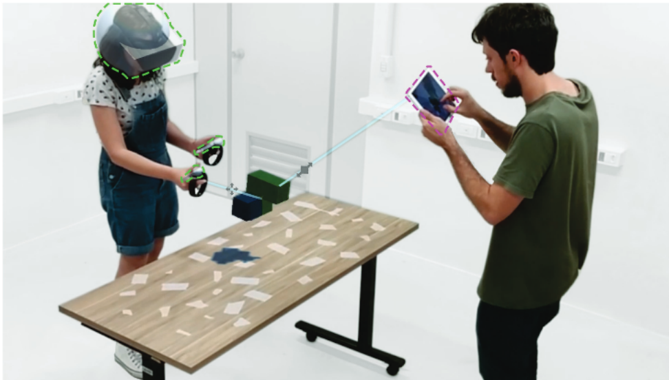
Figure 2.7: A user manipulating a 3D object with VR (on the left), and another user interacting with a 3D object with AR (on the right). Both of them perform rotation manipulation tasks in a synchronous co-located environment.
