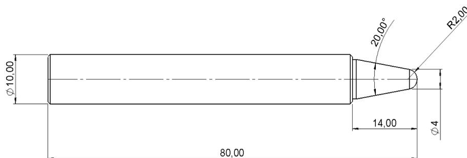
Figura 45 - Ferramenta  $\varnothing$  4mm
