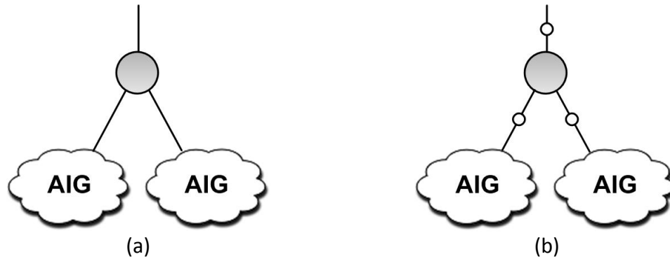
Figure 3.2. The (a) AND operation and the (b) OR operation over two AIGs, generating a new one.
