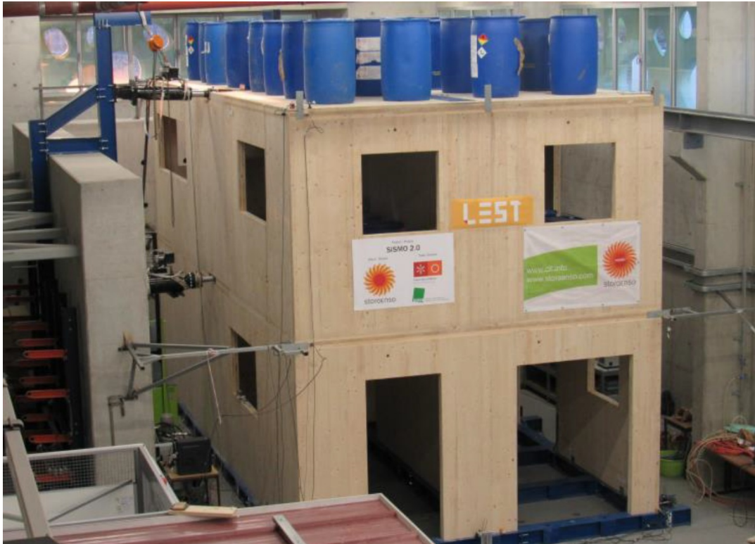
Figure 2.3 – Real scale CLT building, tested Experimental CLT cle at the University of Minho lab facilities. (De MATOS, 2020).
