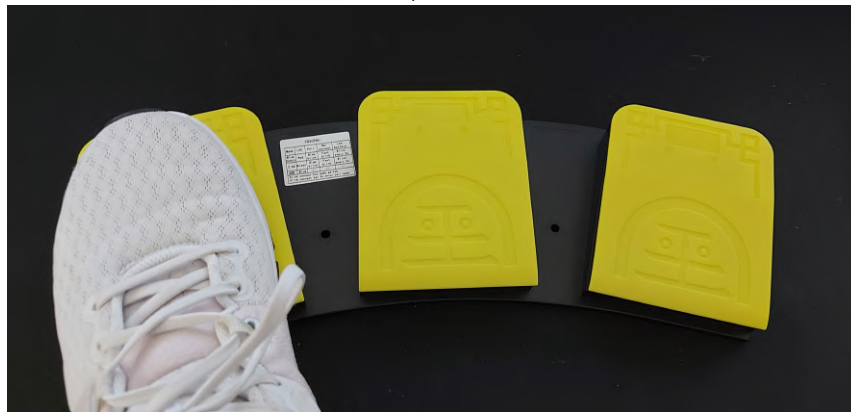
Figure 4.3 – Commercially manufactured wireless foot pedals (we use only two of three inputs).
