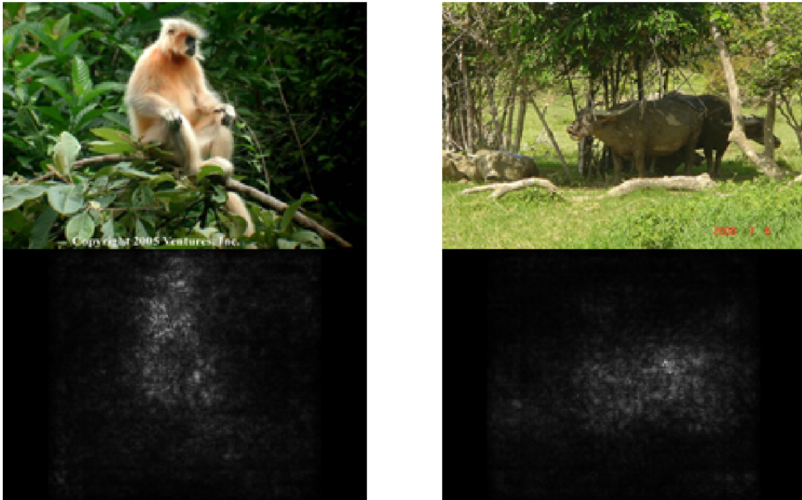
Figure 2.2: Example of class saliency maps to classifications of a monkey and an ox.
