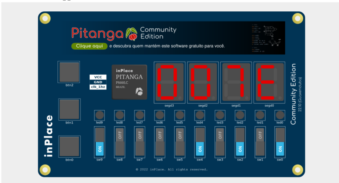
Figure 4.8: The Pitanga virtual board emulating a 16-bit accumulator. The push-buttons and toggle switches are sensitive to mouse clicks.
