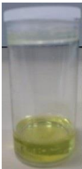
Figure 1 Precursor solution for the production of fibers by electrospinning.
