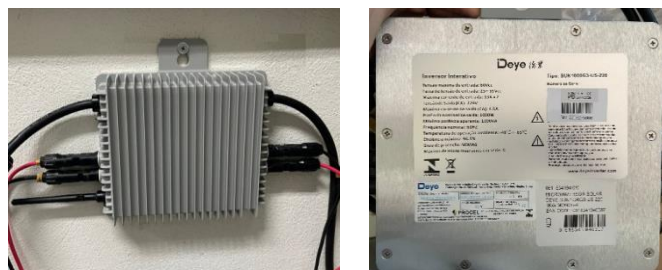
Figura 4: Microinversor Deye (SUN1000G3-US-220)
