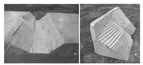
**Figure 18.** Types of machining Styrofoam blocks: A) Detail in the machining of the river channel; B) Variability in the machining of the steps in the same Styrofoam block piece.
