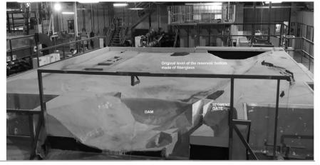
Figure 12. Top view of the reduced Model 02 of SHPP Salto Paraopeba (Fundação Christiano Ottoni, 2013) and physical Model 02, where the fiberglass is already installed.
