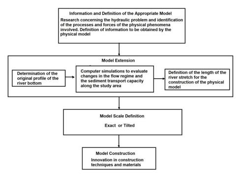
Figure 1. Flowchart of the methodological procedure in the phases of design and model building.
