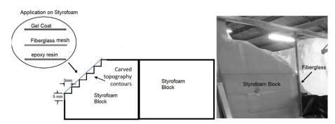
Figure 13. Application of fiberglass over polystyrene blocks (Styrofoam).
