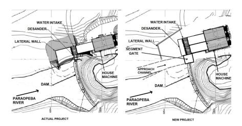
**Figure 2.** Drawing of the project as it is currently (on the left) and the new proposal with the segment gate in the left shoulder pad. (Note: the drawings are illustrative and do not correspond to the original drawings of the project but represent the proposed changes).
