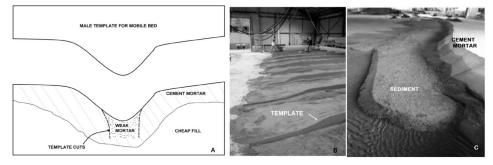
**Figure 17.** The construction process of the morphology in the conventional method: A) Use of templates for the construction of the model (Sharp, 1981); B) Placement of the templates (Water Research Laboratory, 2022); C) Physical model of the mobile bottom (Luo et al., 2018).
