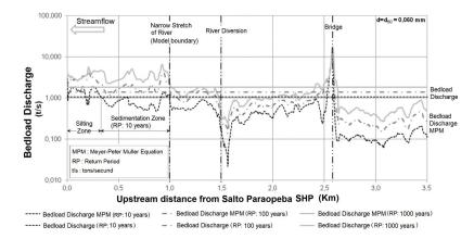
Figure 9. Bedload discharge for 10-yr., 100-yr and 1000-yr recurrence floods using the silted reservoir topography.
