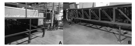
Figure 16. Type of structural base: A) Mobile frame for the undistorted model; B) Fixed frame with tilting system and mechanical jacks for the distorted model.
