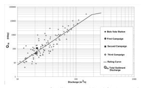
**Figure 5.** Key-curve of sediment considered for SHPP Salto do Paraopeba (Do Vale et al., 2013).
