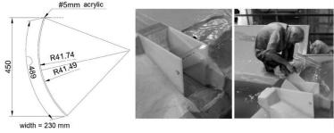
Figure 14. Details of the acrylic segment of the gate and its manual activation.
