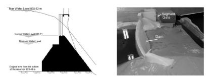
Figure 15. Water levels over the dam (prototype) and detail of the construction of the dam, at the scale of the physical model (executed with a mix of mortar and crushed rubber).
