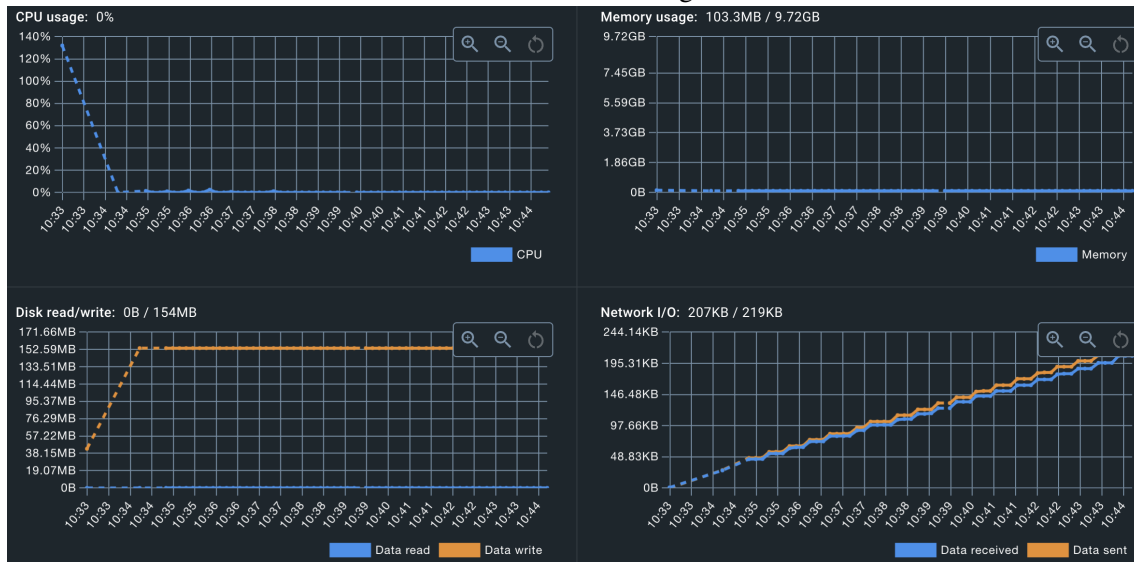
Figure 7.3 – Backend container resources graph demonstrating the CPU, memory, disk read/write and network I/O usage
