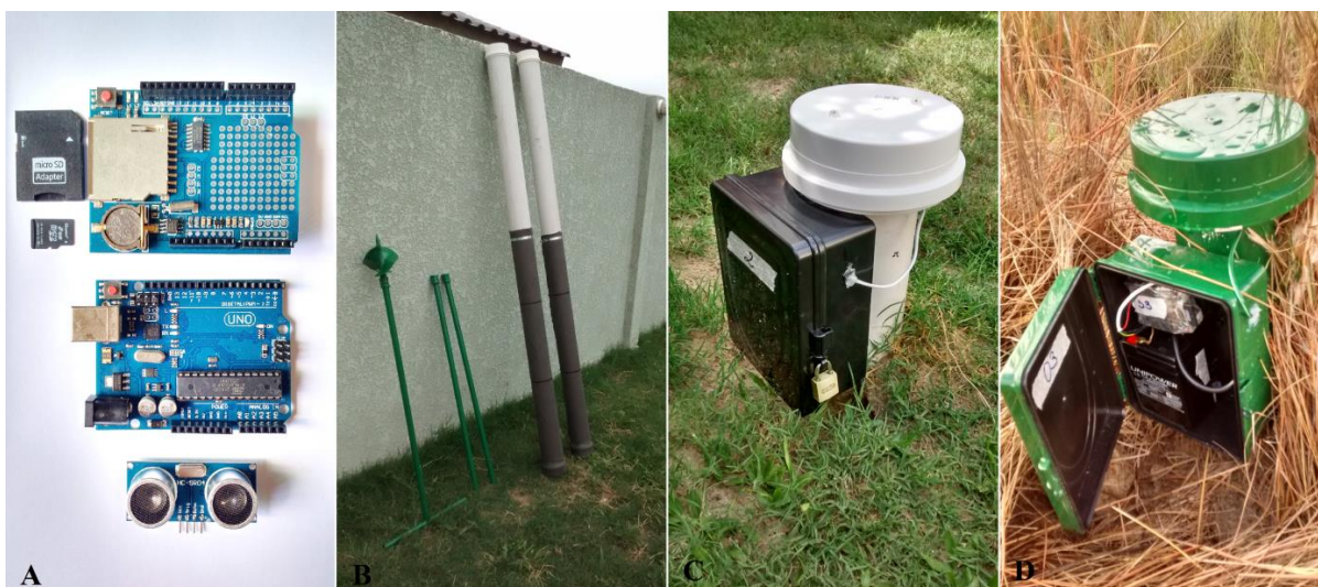
Figure 2: Components of monitoring wells. A) Sensor-system: Arduino microcontroller, microSD card, shield data logger and HC-SR04 ultrasonic module; B) PVC tube perforated and partially covered with geotextile sheet; C) Sensor-system in the urban area; D) Sensor-system in dune swale.
