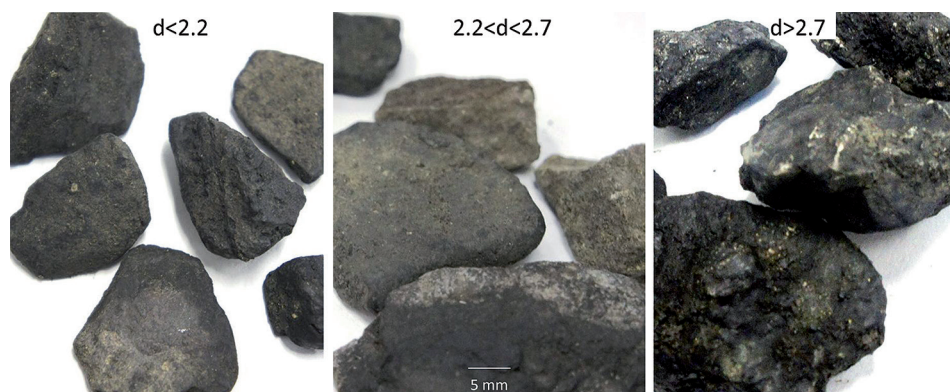
Figure 4 Images of the energetic fraction (d < 2.2), intermediate fraction (2.2 < d < 2.7), and pyrite rich fraction (d > 2.7) of the Bonito seam obtained after densimetric separation.
