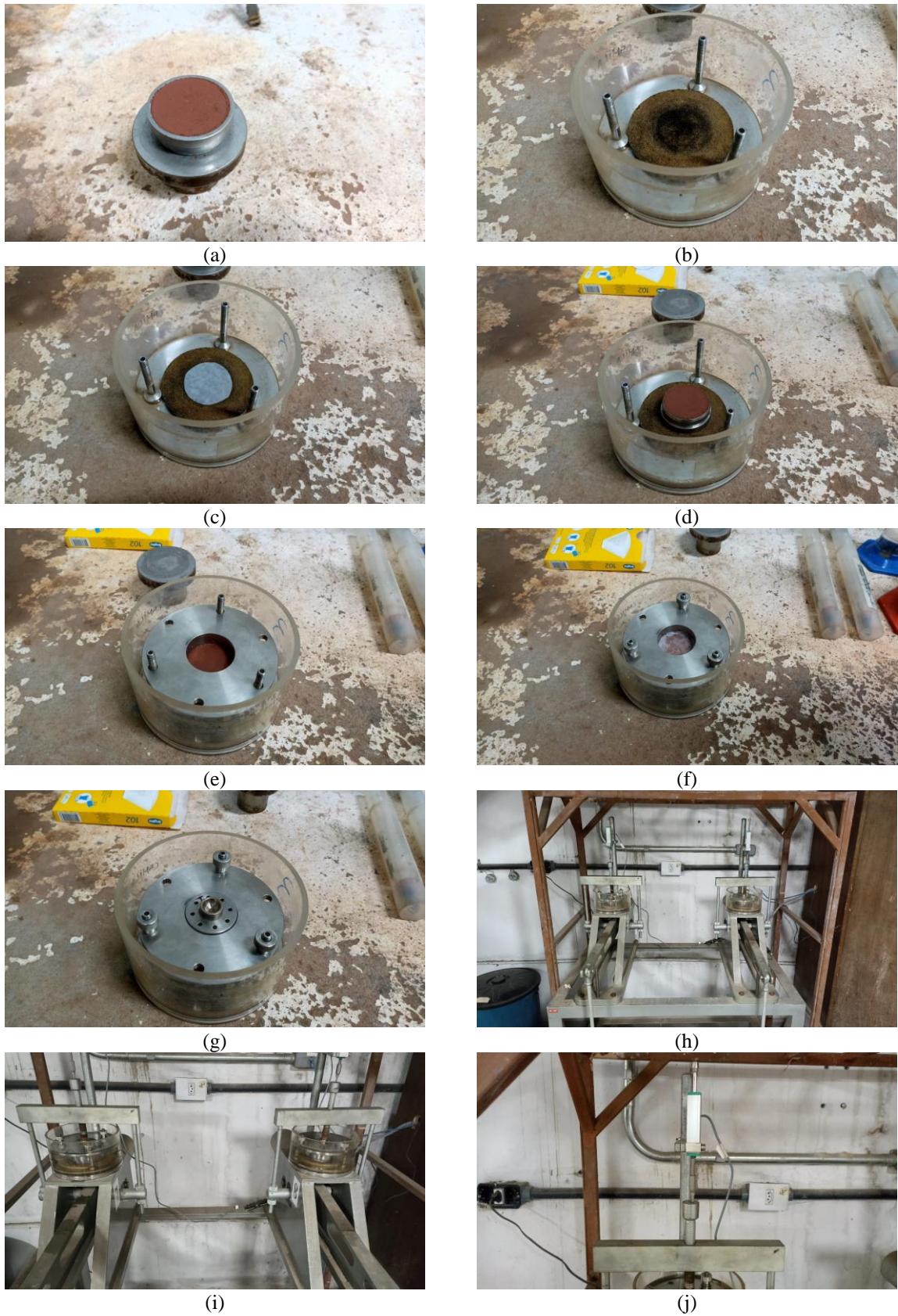
Figure 3.12. Compressibility test: (a) oedometer specimen; (b) chamber and porous stone; (c) bottom filter paper allocation; (d) specimen allocation; (e) chamber ring allocation; (f) bottom filter paper allocation; (g) top cap allocation; (h) general view of the test; (i) saturated specimens; (j) linear variable differential transformer.
