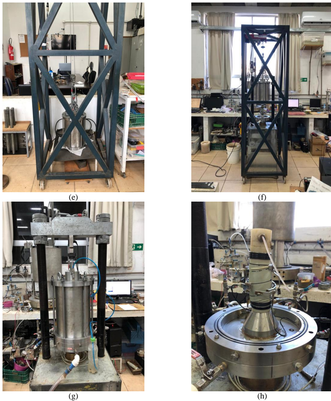
Figure 3.16. High stress triaxial test: (a) latex membrane marking; (b) specimen allocation on the membrane; (c) specimen allocation on the triaxial test; (d) internal sensors allocation; (e) chamber tow; (f) chamber allocation; (g) test disposition; (h) specimen after testing.
