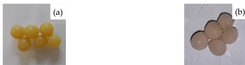
Figure 6. ALDC immobilized in alginate (a)/gelatin (b) particles before and after vacuum drying.
