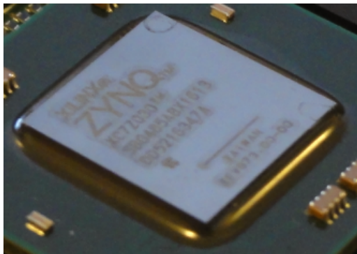
(c) Zynq-7000 XC7Z030 delidded flip-chip
