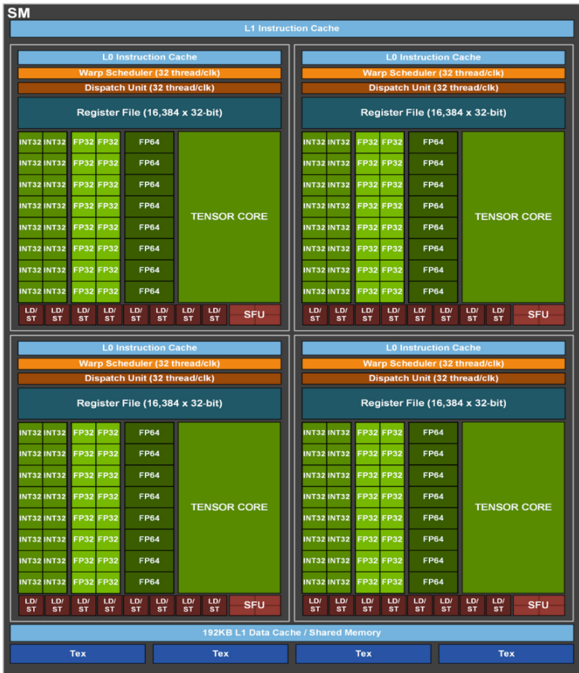
Figure 3.3 – NVIDIA's A100 GPU Streaming Multiprocessor (SM).
