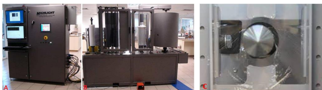
Figure 1: Characterization equipment. (A) Control panel and (B) Analysis board of Highlight Tester®; (C) Illustration of tear propagation resistance analysis (FPT750 - ESTL laboratory)
