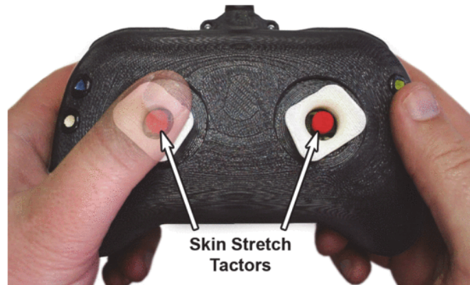
Figure 2.5 – Controller with skin stretch haptic feedback. Guinan et al. (2013)
