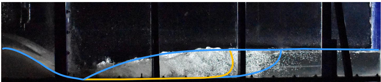
Figure 13.- Roller (yellow) formed for hydraulic jump (blue) with specific flow rate of 0.088 m 3 /s and F_1 = 3.4 . Steinke (2020).
