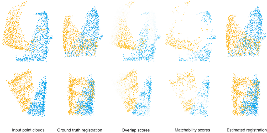
Figure 2.3: Examples of registration using Predator on pairs of clouds from the ModelNet40 dataset (WU et al., 2015). All columns have source clouds in blue and target ones in orange. The overlap and matchability scores are demonstrated as shades of each color. This means that points with a higher score have more saturated colors.
