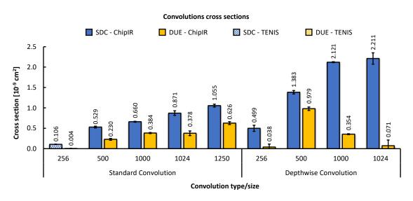
As shown in the Figure above, the SDC cross section increases with the size of the convolution input. Intuitively, this is justified as the systolic array becomes more occupied due to the increasing amount of data that needs to be processed. With more hardware area being actively used, the probability of a neutron hitting the board and causing an error increases.
