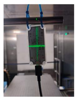
Figure 3.3: The Coral TPU aligned with the high-energy neutron beam at ChipIR
