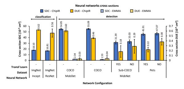
Figure 4.4: Cross sections for the eight CNN configurations that were exposed to highenergy neutrons at Chip IR facility and to thermal neutrons at EMMA facility
