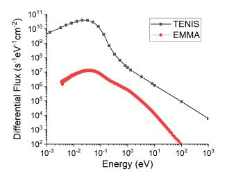
Figure 3.5: Comparison of the neutron energy spectra of EMMA and TENIS
