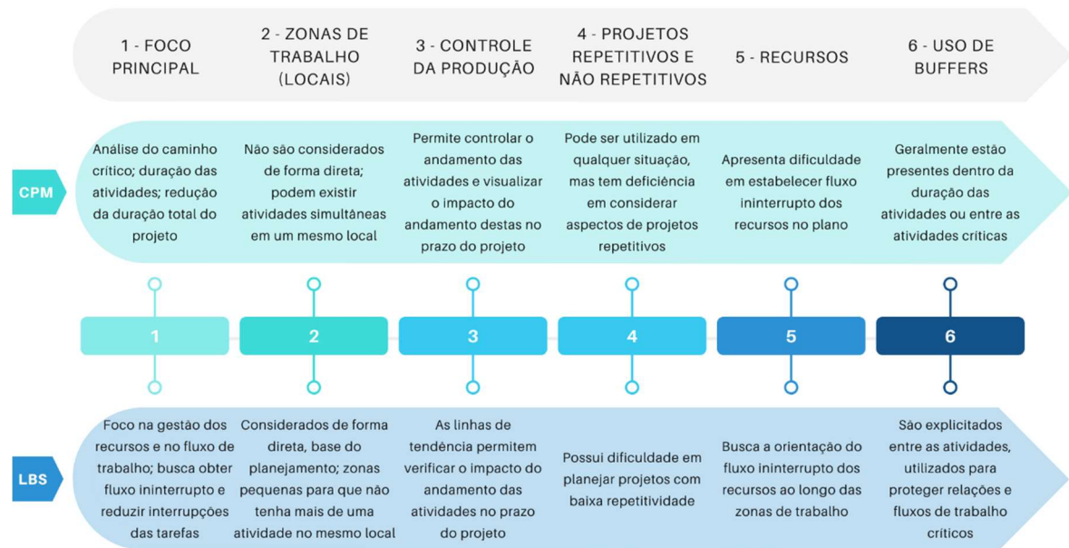
Figura 1 - Comparativo entre CPM e Location-Based Management System (LBS).
