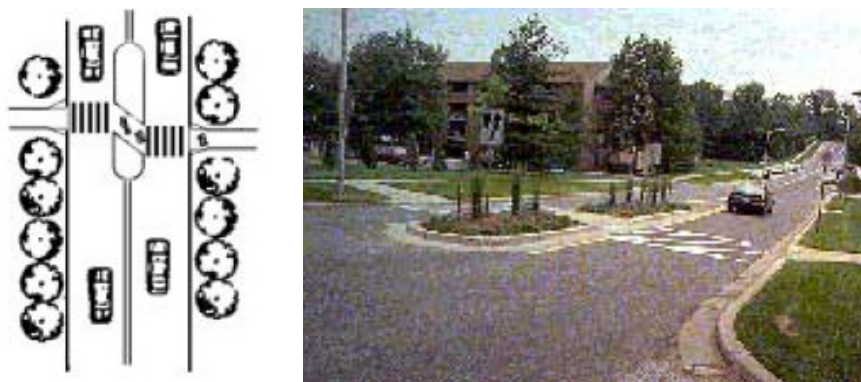
Figura 10: ilhas de travessia (FEDERAL HIGHWAY ADMINISTRATION, 2002)
