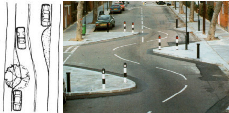
Figura 9: chicanas (FEDERAL HIGHWAY ADMINISTRATION, 2002)
