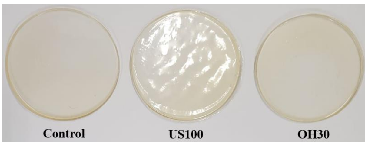
Figure 6 - Visual appearance of gelatin-based films produced by different technologies.
