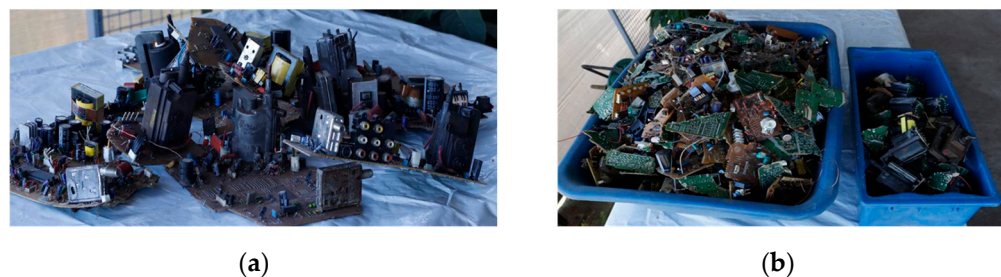
Figure 1. (a) Raw PCBAs samples. (b) Samples after dismantlement: PCBs (left) and voltage and flyback transformers (right).
