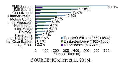
Figure 1. Time percentage of each stage in the video encoding process.
