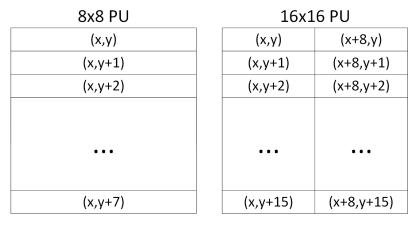
Figure 4.2: Requests for  $8 \times 8$  and  $16 \times 16$  PUs considering a word size of 8 bytes.
