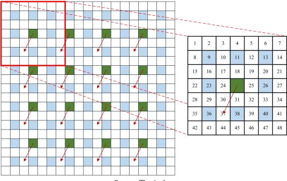
Figure 2.7: FME fractional pixels window for a  $4 \times 4$  PU.
