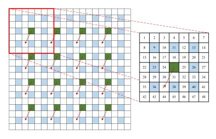
Figure 8. FME fractional pixels window for a  $4 \times 4$  PU.
