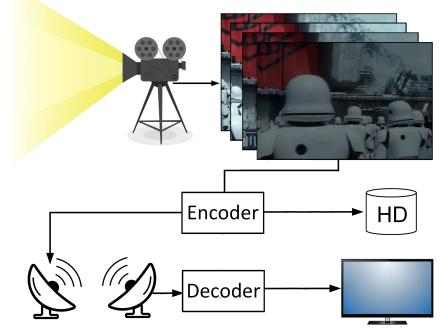
Figure 2.1: Simplified scheme of encoding and decoding in video transmission.
