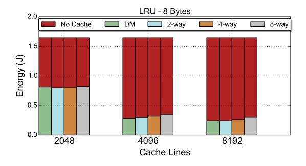
Figure 5.4: Energy results of the memory hierarchy (8-byte word size).
