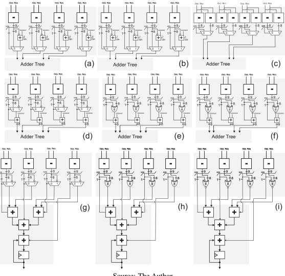
Figure 4.3: Absolute differences operation architectures.
