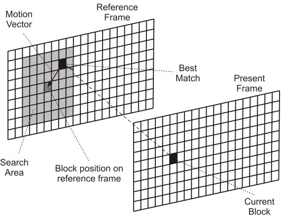
Figure 2.4: Generic search in a previously coded frame.
