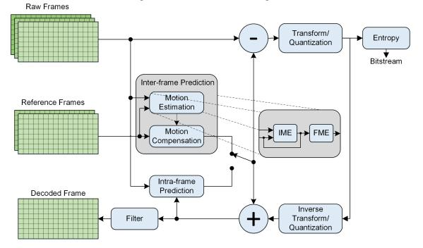
Figure 2.2: Video encoder diagram.
