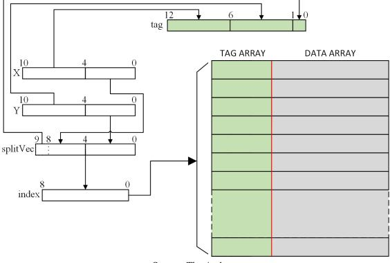
Figure 4.1: Index and tag formation based on the proposed model.
