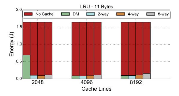
Figure 5.6: Energy results of the memory hierarchy (11-byte word size).
