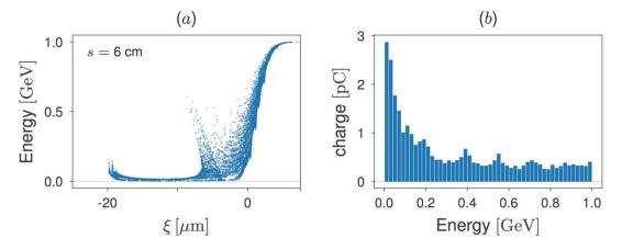
**Figure 1.** (**a**) The EuPRAXIA 1 GeV beam longitudinal phase space and (**b**) energy spectrum, both plotted after 6 cm propagation in plasma.
