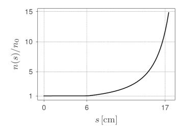
**Figure 2.** A tailored plasma density profile designed to eliminate the re-acceleration of particles in the bunch tail in the EuPRAXIA 1 GeV beam. The plasma density exhibits uniform behaviour until s = 6 cm, followed by a non-linear growth that reaches a 10 times higher density at s = 16.8 cm compared to the former uniform plasma density.
