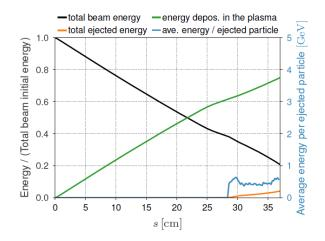
**Figure 8.** The energy plots as a function of propagation distance in plasma, for the plasma density profile shown in Figure 6 for the EuPRAXIA 5 GeV beam.
