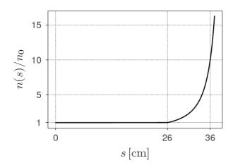
**Figure 6.** A tailored plasma density profile designed to eliminate the re-acceleration of particles in the bunch tail in the EuPRAXIA 5 GeV beam. The plasma density exhibits uniform behaviour until s = 26 cm, followed by a non-linear growth that reaches a 15-fold higher density at s = 36 cm, compared to the former uniform plasma density.
