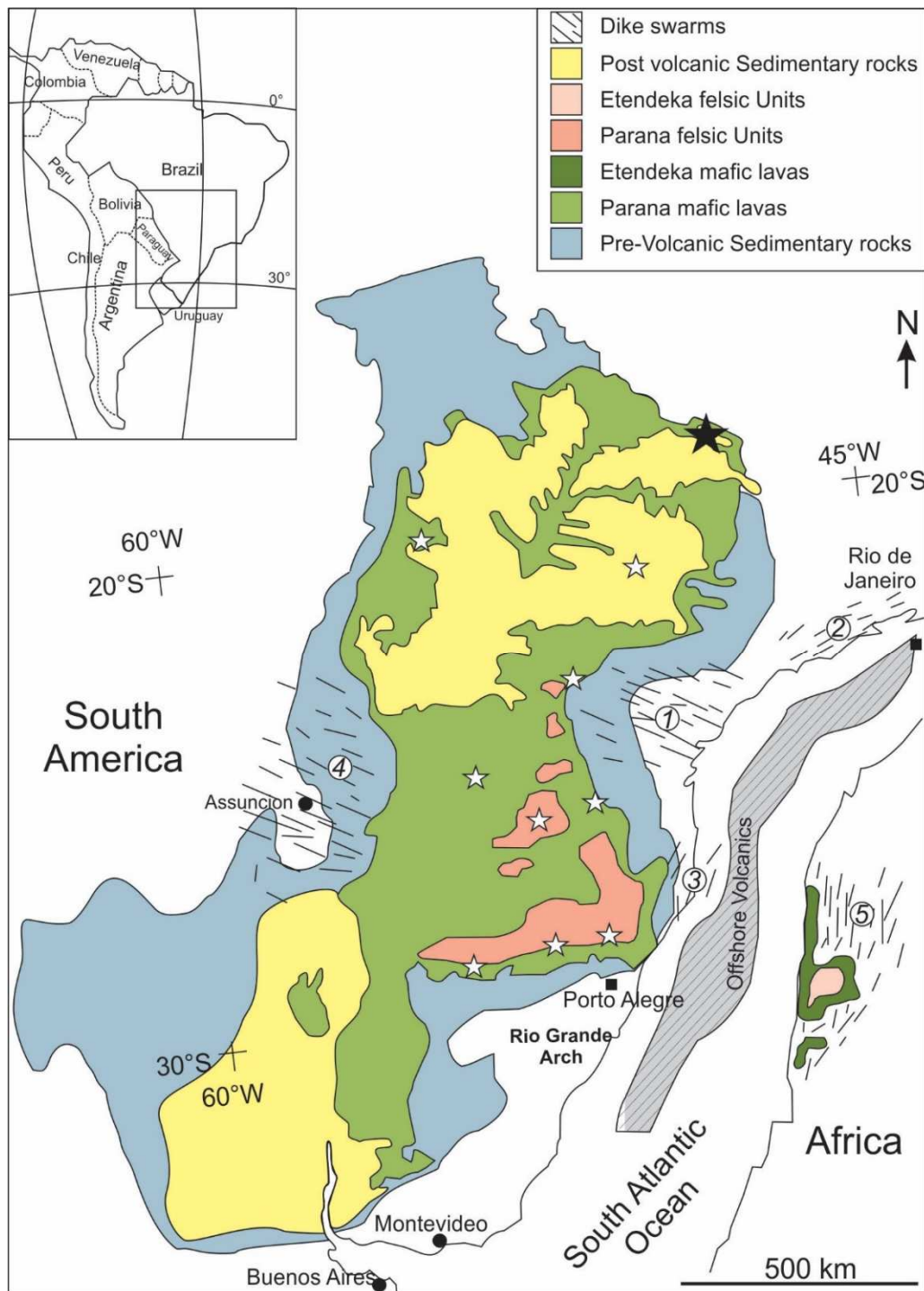
Fig. 32: Geological map of the Paraná Basin (modified after Hawkesworth et al., 2000; Peate et al., 1992; Rossetti et al., 2018; Stewart et al., 1996). Dike swarms: 1 – Ponta Grossa; 2 – Santos-Rio de Janeiro; 3 – Florianópolis; 4 – Paraguay; 5 – Skeleton Coast. Stars represent pillow lava and peperite occurrences. The black star highlights the location of the study area.
