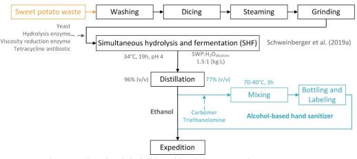
Figure 2. Ethanol and alcohol-based hand sanitizer production processes Source: The authors themselves
