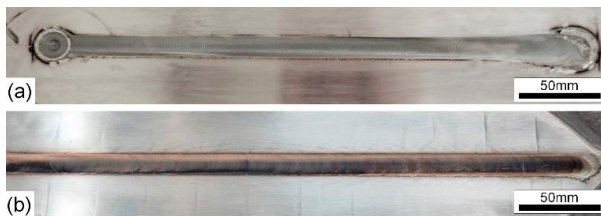
Fig. 1 (a) 1st FSW pass on API X65 steel side. (b) 2nd FSW pass on Inconel 625.
