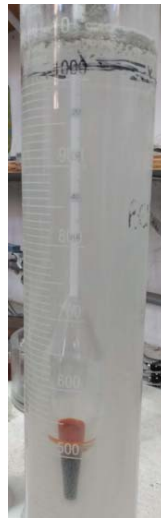
Figure 3.3: Hydrometer inside the glass cylinder.
