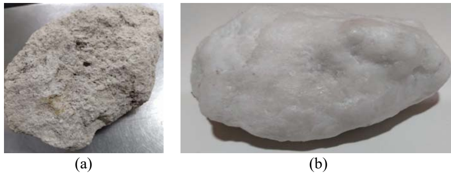
Figure 3.10: (a) intact soil sample; (b) soil covered by wax.
