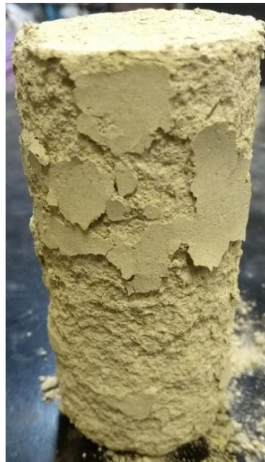
Figure 3.24: Typical behaviour stabilized soils with a high mass loss after wetting and drying durability tests.
