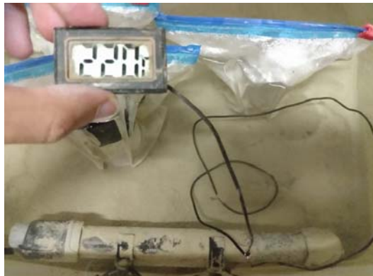
Figure 3.22: Water curing tank with controlled temperature.
