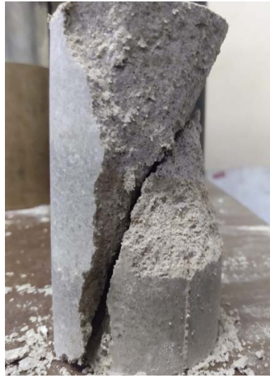
Figure 3.26: Typical shear surface for medium-high cemented soils in unconfined compressive tests.
