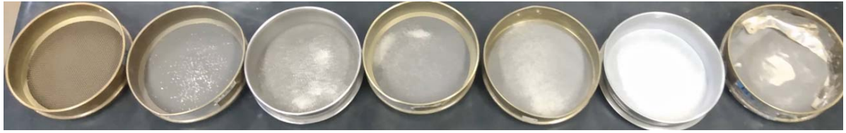
Figure 3.2: Sieves from left to right: 2.000 (#10), 1.180 (#16), 0.600 (#30), 0.425 (#40), 0.250 (#60), 0.150 (#100) and 0.075 mm (#200).
