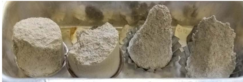
Figure 3.27: Soil portion taken for the samples moisture determination after failure.
