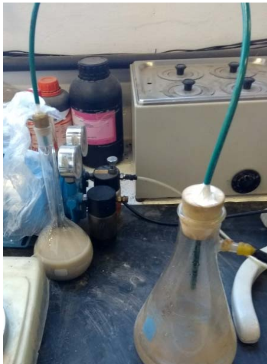
Figure 3.7: Vacuum pump for the pycnometer analysis.
