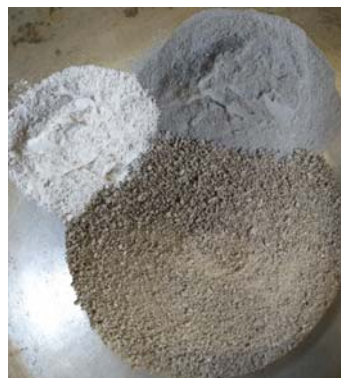
Figure 3.21: Soil, fly ash, and calcitic lime (yellow-brown, dark gray and white color, respectively) prepared for molding.
