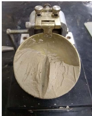
Figure 3.5: Soil liquid limit test with Casagrande's device.
