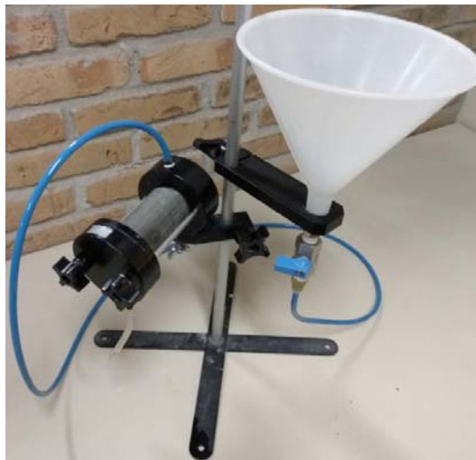
Figure 3.19: Pinhole test equipment.
