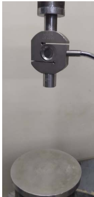
Figure 3.25: Unconfined compression equipment with 10 kN load cell.
