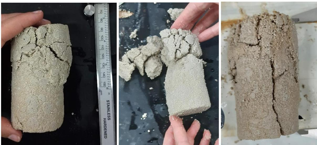
Figura 4.22: Rupturas das amostras SA (a) 20 kPa (b) 60kPa (c) 100 kPa.
