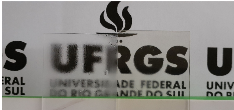
Fig. 8. Subjected to water vapor, from left to right, bare glass and coated samples show the antifogging property of the latter.
