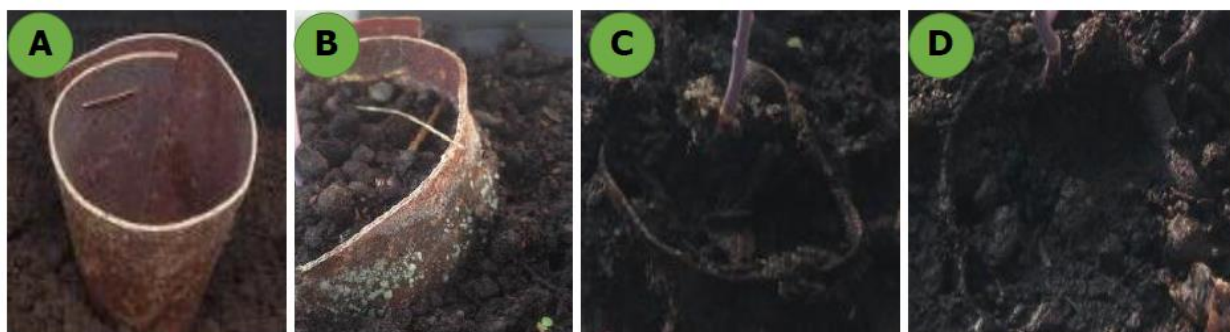
Figure 2 – Degradation of apple bagasse films to F2 formulation: (a) prior to the beginning of the degradation process, (b) 30 days, (c) 45 days and (d) 60 days after
