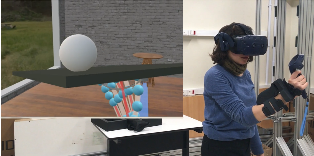
Figure 2.4: Participant carrying the virtual tray (left side) with the haptic feedback provided by the wearable device.
