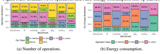
Figure 5.26: Breakdown of operations and ALU energy consumption into op classes.
