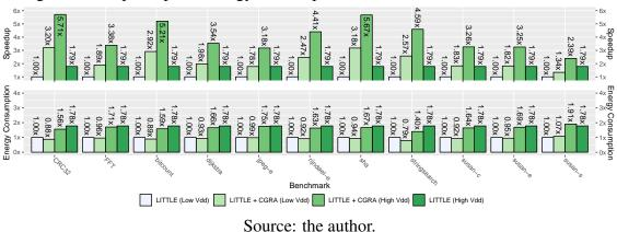
Figure 5.22: Speedup and energy consumption in a LITTLE core and in MuTARe.
