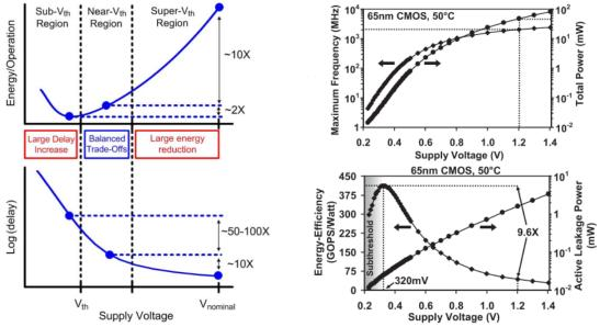
Figure 2.12: Effects of voltage scalability in delay and energy consumption.
