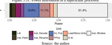
Figure 5.31: Power distribution in a superscalar processor.
