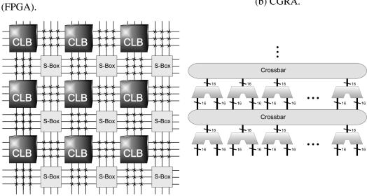
Figure 2.3: Comparison between an FPGA and a CGRA. Field-Programmable Gate Array (b) CGRA.
