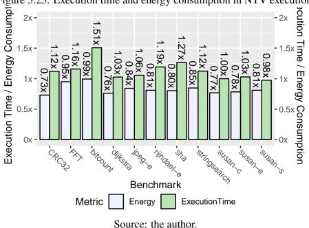
Figure 5.25: Execution time and energy consumption in NTV execution.
