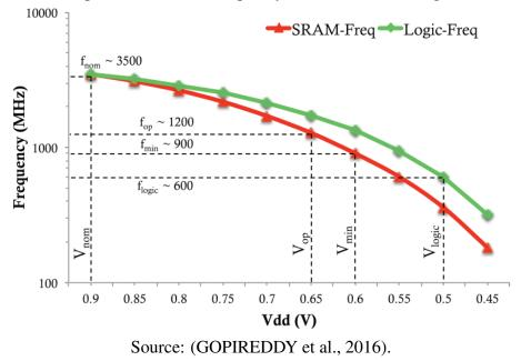
Figure 2.13: Impact in maximum frequency as  $V_{dd}$  is lowered (logic vs memory).
