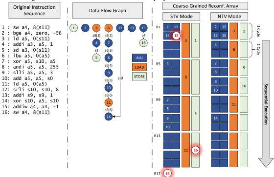
Figure 4.4: Accelerated chains of memory operations in NTV-MuTARe.
