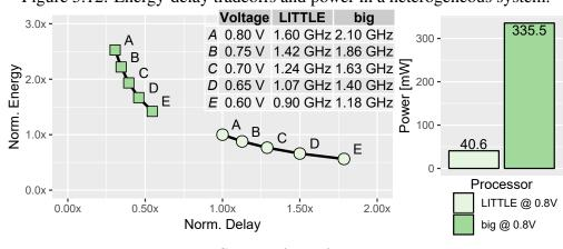
Figure 5.12: Energy-delay tradeoffs and power in a heterogeneous system.
