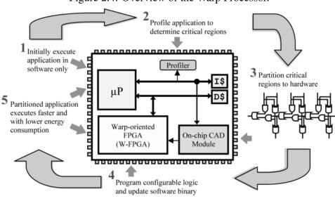
Figure 2.4: Overview of the Warp Processor.
