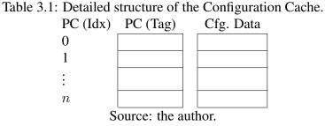
The size of each configuration varies according to the size of the CGRA, so that should be taken into account during design to balance the configuration load times with the bandwidth offered by the cache. For instance, in sigle-issue, small pipeline processor the configuration load time is critical to achieve high performance. In superscalar cores, however, with larger instruction windows, it is typically less critical to load configurations fast as a higher number of instructions will execute.
