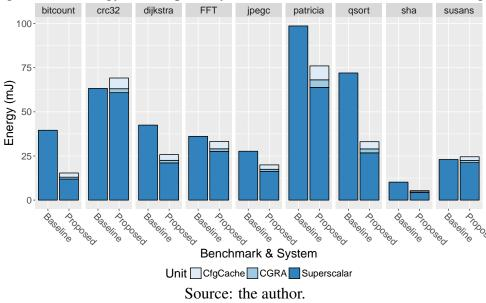
Figure 5.11: Energy consumption by each benchmark with the 30-level design.
