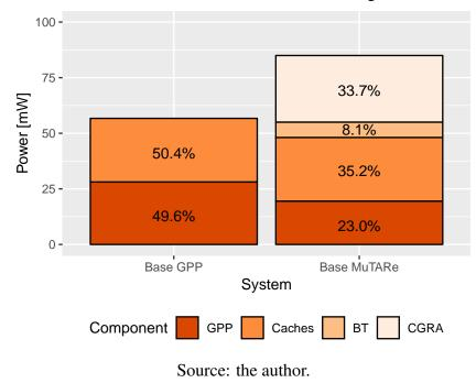
Figure 5.21: Power breakdown with and without reconfigurable acceleration.
