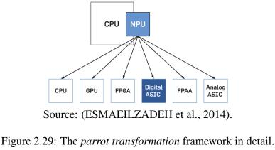
Figure 2.28: Design space for implementing an NPU.
