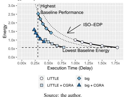
Figure 5.14: Energy-Delay curves for different execution units and DVFS levels.
